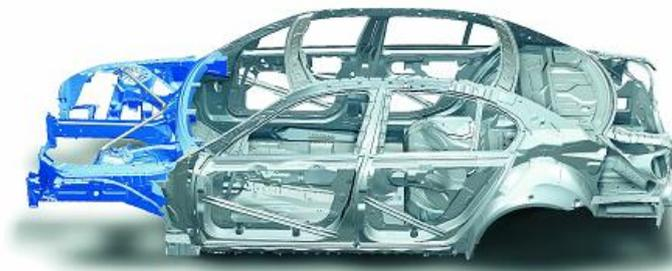
**BMW 5xx model E60 with an aluminium front section built from 2003 to 2010
