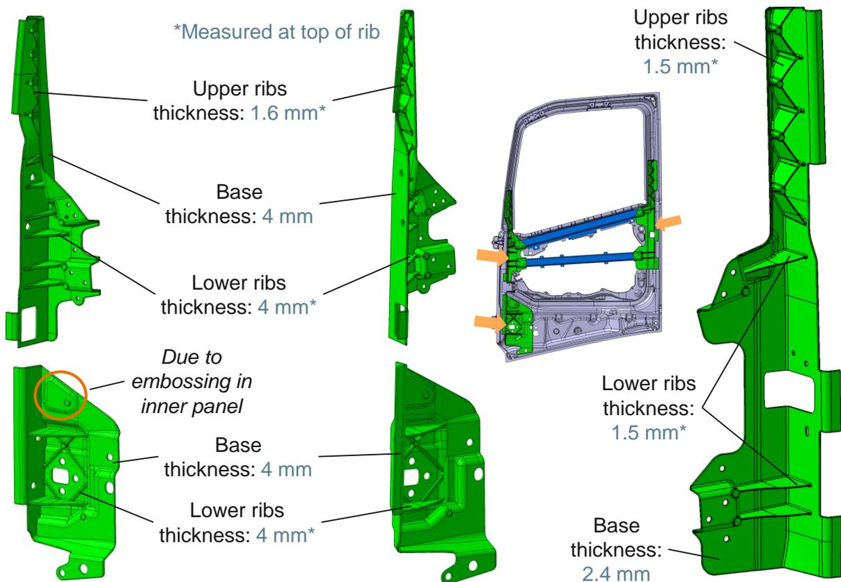
Fig. 4-3: Aluminium Door Concept V1.6 - Casted Reinforcements
