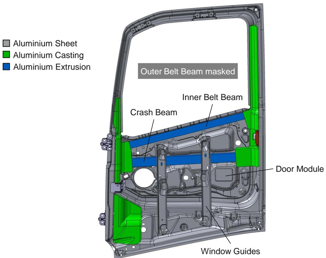
Fig. 4-1: Design spaces for casting & extrusion applications (outer panel masked)
