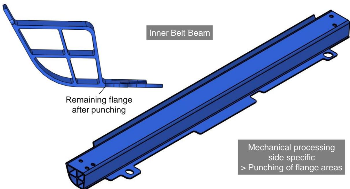
Fig. 4-4: Inner Belt Beam geometry for left door (driver's door) - V1.6
