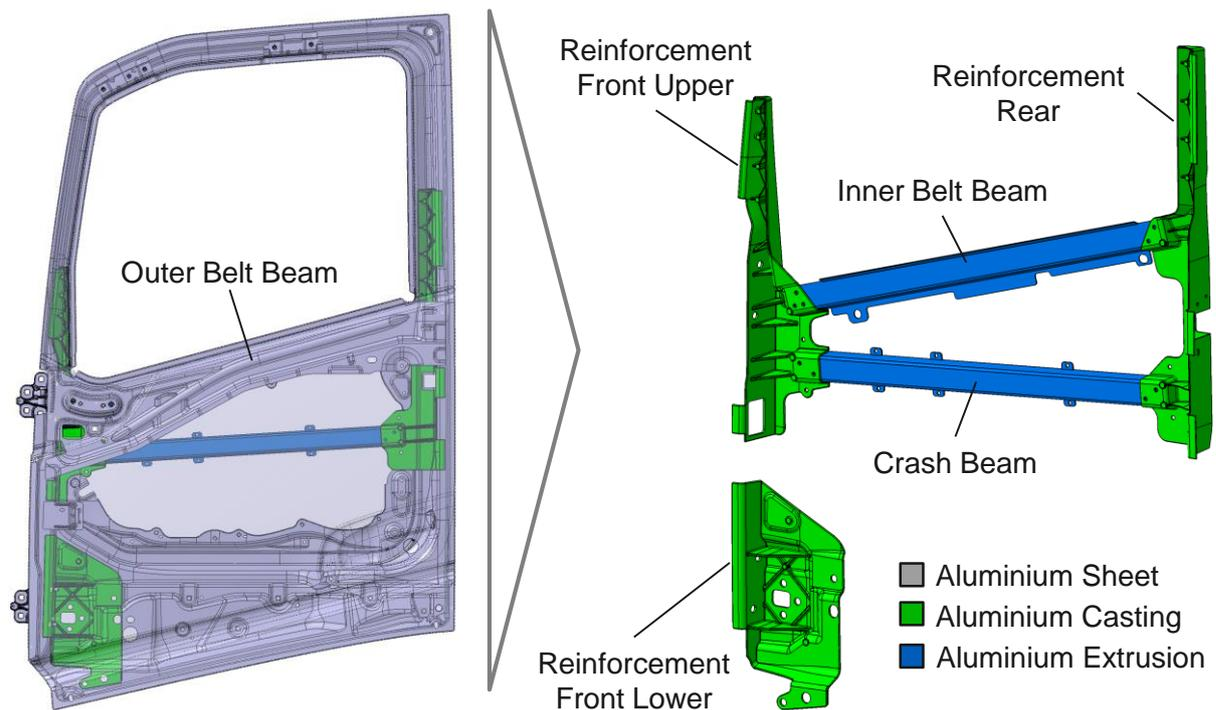
Fig. 4-2: Aluminium Door Concept V1.6
