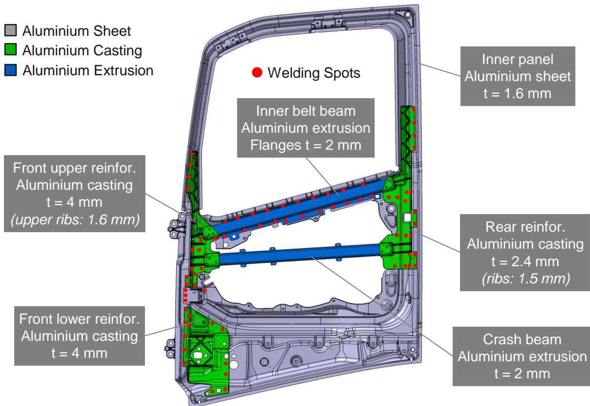
Fig. 5-1: Components to Inner Panel - Overview joining constellations
